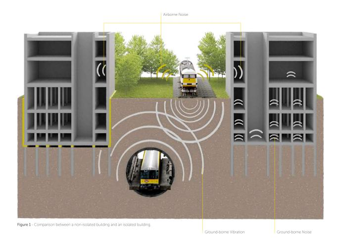
Integrating an economical and sustainable vibration control into a building requires the introduction of a Building Base Isolation solution in the early design phase of a project. In close collaboration with the structural and architectural design teams, a decoupling strategy is proposed. This decoupling level, commonly called the "vibration cut" will include the BBI solution and depends on:
