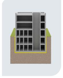
Figure 4.1 - Decoupling the entire building from the soil
