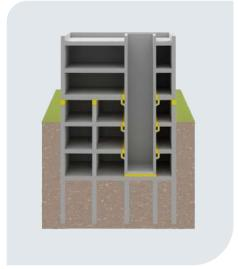
Figure 3 - Isolation of the building considering the elevator pit
