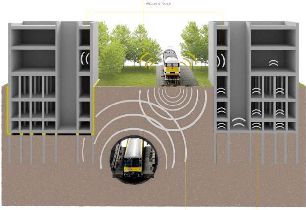
Figure 1 - Comparison between a non-isolated building and an isolated building.
