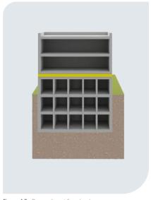
Figure 4.3 - Decoupling at floor level
