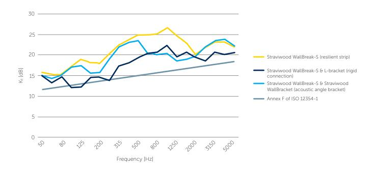
Image 2 - Total vibration reduction index (K,) of T-junction with different connectors compared to standard values.
