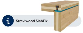
The flood/roof-slab connection can be acoustically decoupled using the Straviwood SlabFix, a customizable design available upon request.
