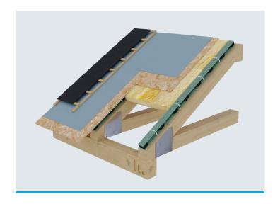
Image 6 - Stravifloor Batten on wood frame – roof.
