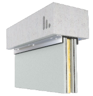
Stravilink RHD (Resilient Head Detail)
