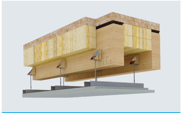
Image 5 - Stravifloor lightweight floating floor combined with a dropped ceiling using Stravilink IJH-P hangers.
