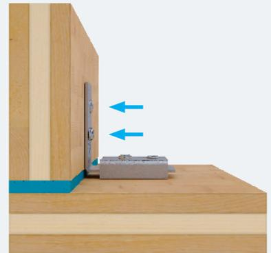
Image 9 - Straviwood WallBracket installation steps, showing pre-compression system, designed to avoid over-compression.
