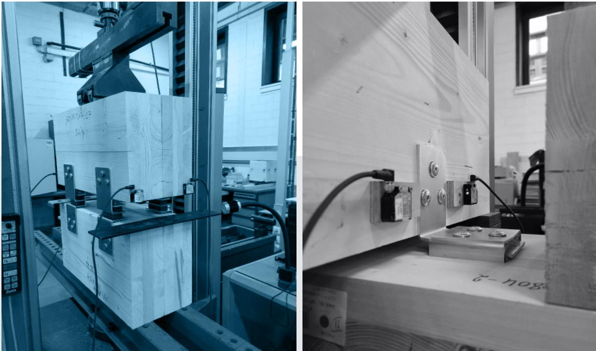
**Image 3** - Mechanical strength test Straviwood ModuLink (bracket for structural joints) in compression (left image) and Straviwood WallBracket (angle bracket for structural joints) in uplift tension (right image).
