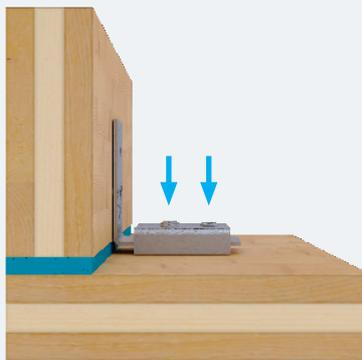
3 - Drive screws on the bare plate side
