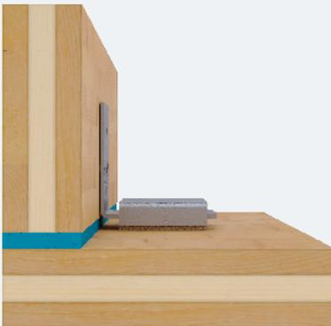
2 - Drive screws on the isolator side until the stabilizer touches wood
