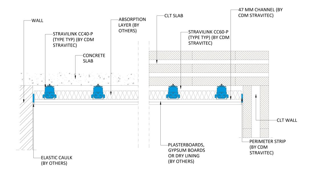
Legend First submission Revision Description Drawing based on cdm. stravitec STRAVILINK CC60-P (CEILING WITH I REDUCED VOID) Typical Cross Sections - Stravilink CC40\_60-P-04 Scale: 1:5 Drawn: ERA 03/02/2025 Format: Design: ERA **⊕** ⊕ A3 Check: MRO
