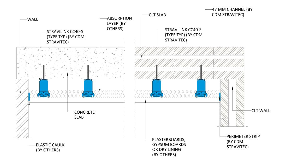
Legend First submission Revision Description cdm. stravitec Reutenbeek 9-11 B-3090 Overijse Belgium PH: +32 2 687 79 07 info@cdm-stravitec.com www.cdm-stravitec.com STRAVILINK CC40-S (CEILING WITH I REDUCED VOID) Typical Cross Section - Stravilink CC40\_60-S (EU)-04 Scale: 1:5 Drawn: 31/01/2025 Design: ERA **⊕** ⊕ A3 Check:
