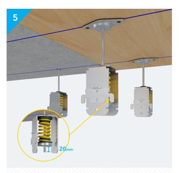
Slide the hanger down. Ensure that no more than 20 mm of the rod extends below the spring steel cap to prevent rigid contact with the channel that will be installed next.
