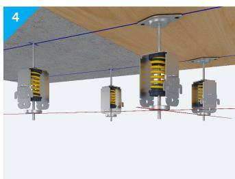
Set the position of the hangers and, consequently, the ceiling by leveling the spring steel cap using a laser.
