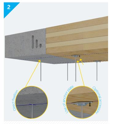
Fixing devices should be used that are suitable for the ceiling material type and load capacity.
