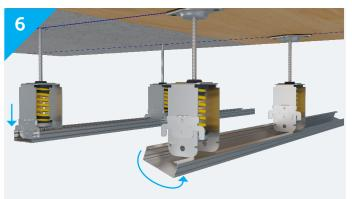
Snap the metal profile into place and slide the safety clip down.
