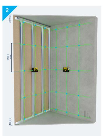
Laser level in the vertical and horizontal directions for Stravilink QRC layout and mark centers.
