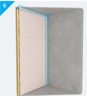
Ensure no rigid contact with the surroundings to prevent acoustic bridging. Use non-setting mastic to seal.
