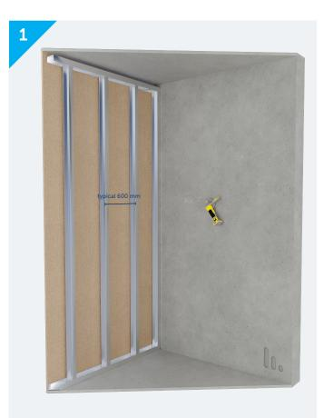
Ensure the wall or stud is level and free of protrusions, masonary may need grinding.
