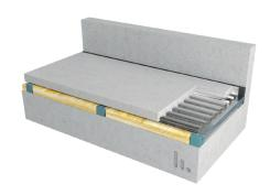
Perimeter Strip can be applied between suspended ceilings and adjacent walls, thereby acoustically decoupling the drop ceiling from its surroundings.
