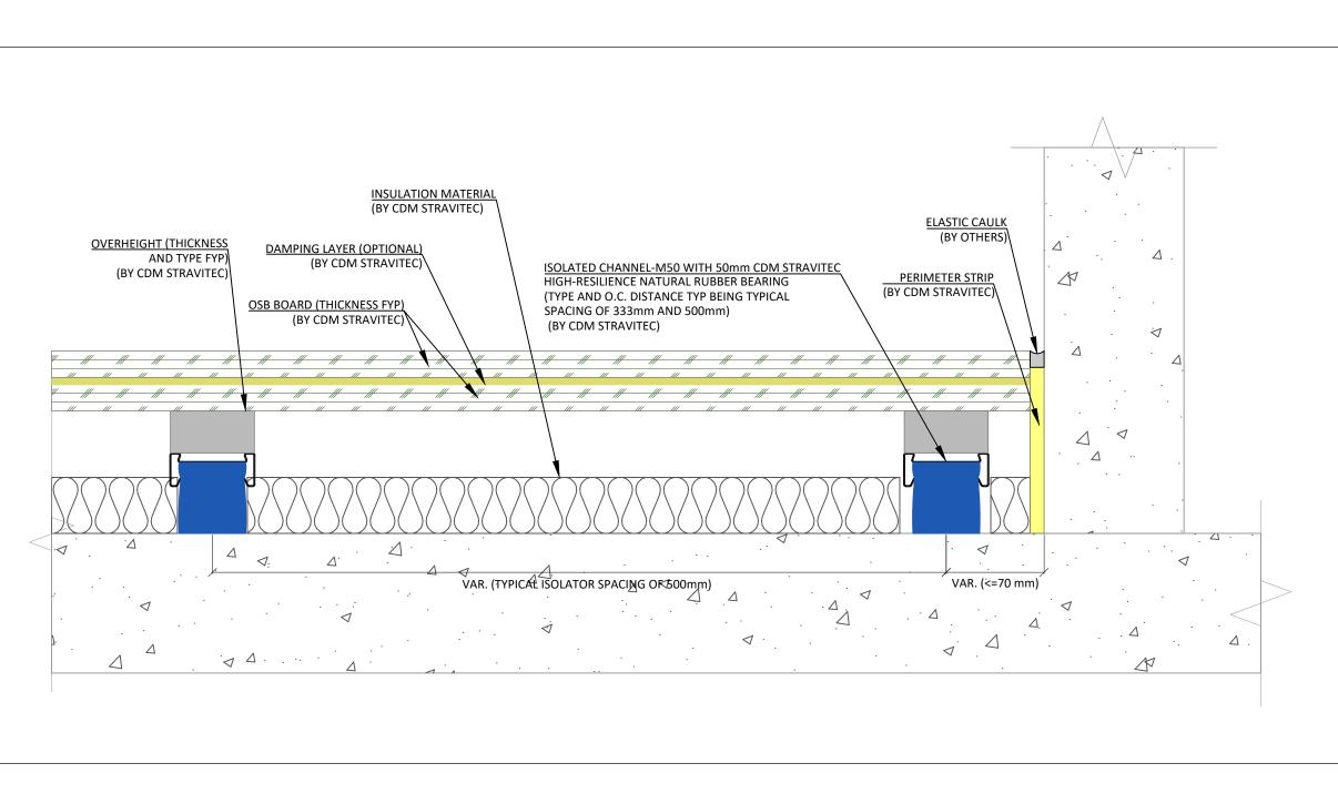
2. A rigid connection should be avoided between the floating slab and all vertical elements (as walls, columns, ...) by adding a void or a layer of lateral isolation between the isolated slab and the vertical element. For more detailed information ask for Stravifloor Channel Installation Manual. Legend
