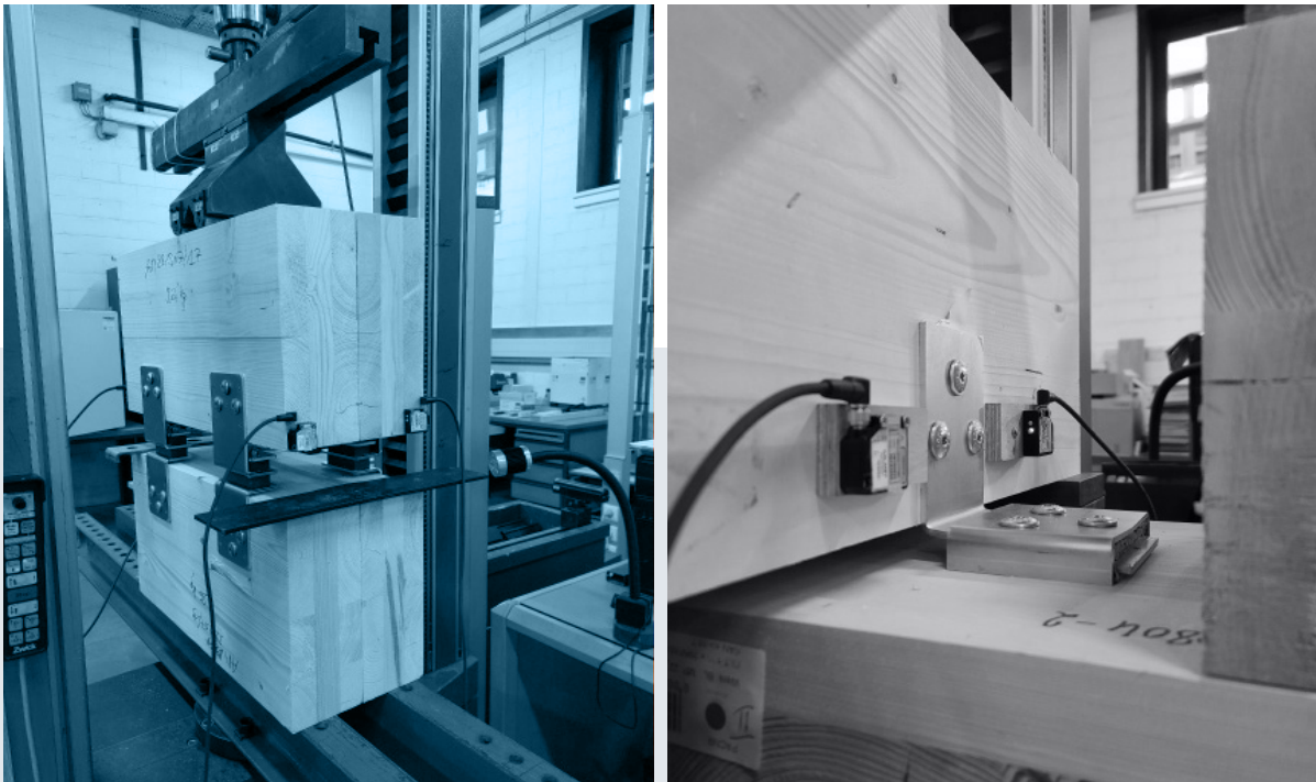
Image 3 - Mechanical strength test Straviwood ModuLink (bracket for structural joints) in compression (left image) and Straviwood WallBracket (angle bracket for structural joints) in uplift tension (right image).
