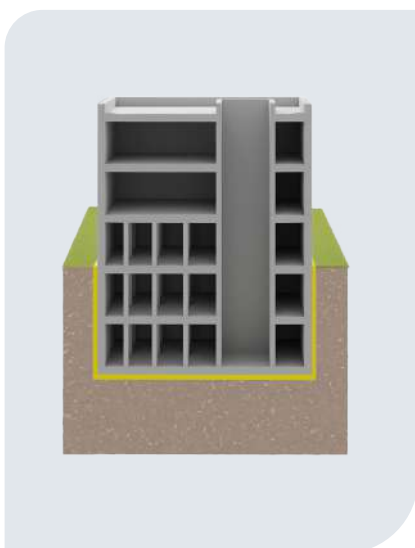
Figure 4.1 - Decoupling the entire building from the soil
