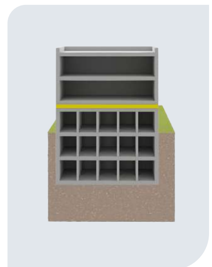
Figure 4.3 - Decoupling at floor level
