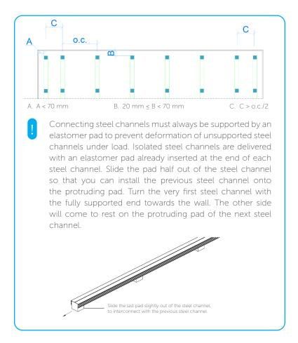
The use of a steel channel around the perimeter of the room is not necessary unless it is known that there will be significant loads in this area i.e. dumbbell racks or other heavy equipment.
