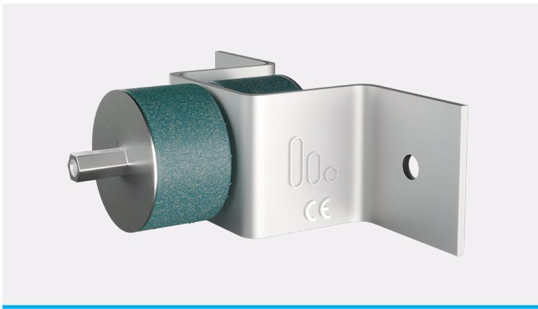
Stravilink WH, resilient wall ties enable walls to be mechanically tied together without rigidly connecting them. Walls can be either stud walls (via bolt end) or brick block walls (via hooked end).
