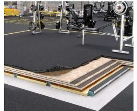
! Stravigym GympactTile can be used as impact absorption layer in a Stravigym XP system.
