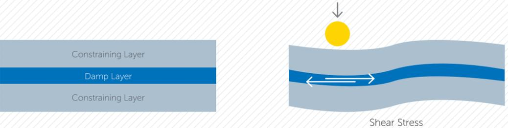
The dips in the resonance and coincidence-controlled region are mitigated by well-known CLD (constrained layer damping) techniques with highly damping, viscoelastic acoustic membranes – Damping Layer.
