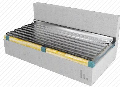
The decking sheets can also be laid in stretcher bond. They must be laid at right angles across the isolated channels, meaning that the profiled section of the decking sheets must be perpendicular to the isolated channels.
