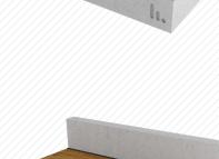
If the Stravitec Channel floating floor system is a different height to the surrounding structure an edge profile will be required. If a rigid edge profile is used ensure that the height of it is less than the height of the total floor system so that it does not make contact with the supporting floor. After deflection [(floor system height - edge profile height) > (deflection + creep)].
