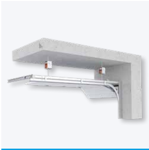
Figure 8 - Depiction of an elastic suspension system designed for sliding garage doors and their accompanying motor, featuring Stravilink PHR. This setup is further enhanced by employing Stravimech Fix for the elastic attachment of the rails.
