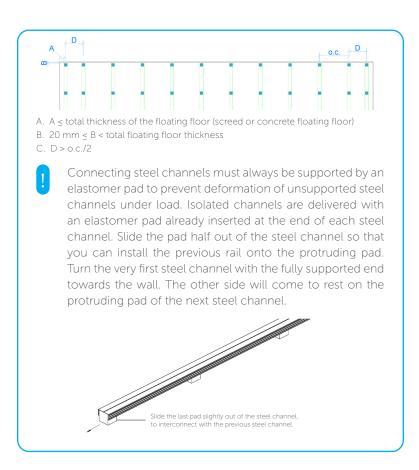
The use of a steel channel around the perimeter of the room is not necessary unless it is known that there will be significant loads in this area i.e. dumbbell racks or other heavy equipment.
