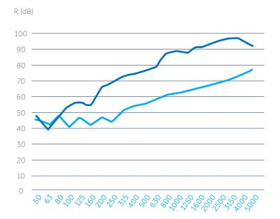
R system with 4.5Hz springs and 150 mm concrete floating slab 50 mm air void
