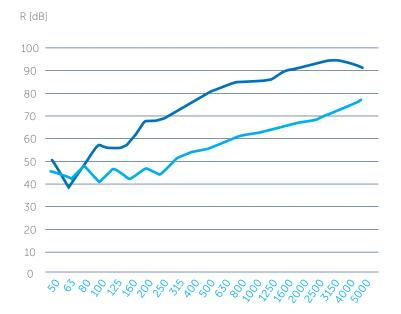
R system with Pad-X50 and 150 mm concrete floating slab 50 mm air void
